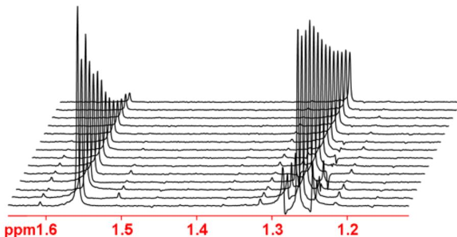
$^1\text{H}$  spin-echo experiments of ethylbenzene (0.1%) in  $\text{CDCl}_3$  at 400 MHz. The residual water peak (left) relaxes faster than that of the methyl (right).
