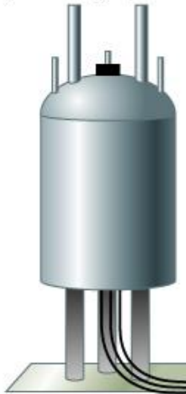
Sample tube spins within the probe coils in the hollow bore at the center of the magnet.
