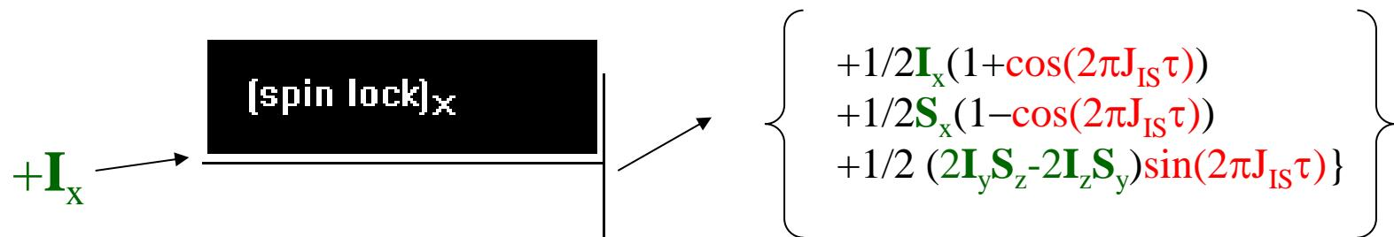
In conclusion during an  $SP_x$  lock  $+I_x \sin(\Omega_I t_1) \cos(\pi J_{IS} t_1)$  and  $+S_x \sin(\Omega_S t_1) \cos(\pi J_{IS} t_1)$  evolves as follows (6 tems in total):
