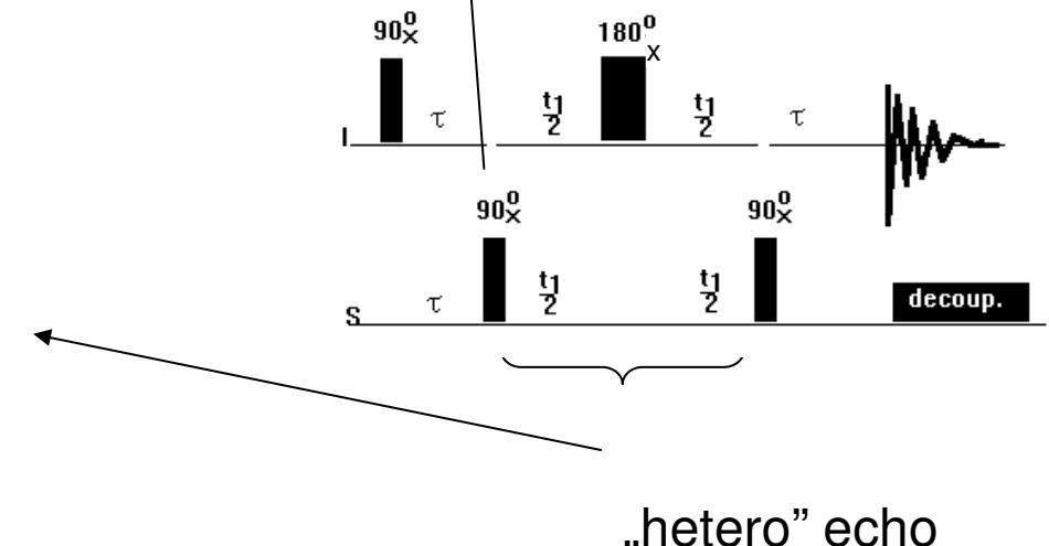
The latter Hemiltonians are of a refocusing module; " ----1/2t<sub>1</sub> ---- 180°<sub>x</sub> ----1/2t<sub>1</sub> ---- ,,. During a „heteronuclear echo” the heteronuclear coupling (**JS**) doesn't evolve and chemical shift doesn't evolve.
