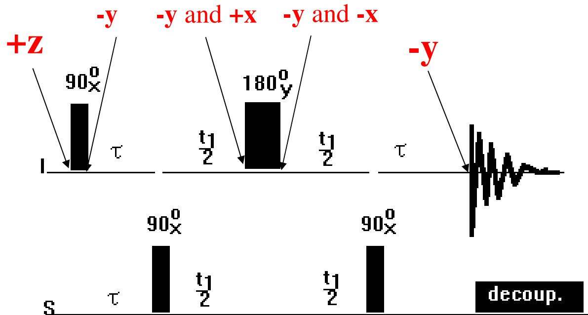
What is happening with the bulk water during the HSQC pulses? If  $\tau+t_1/2 = \Delta$ , then
