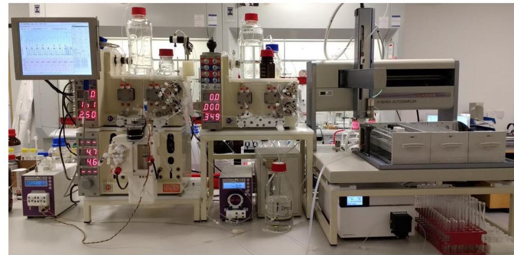
Figure 1 – The CF-SPPS setup, consisting of two R2 pump modules, one R4 reactor module, autosampler and in-line UV detector.
