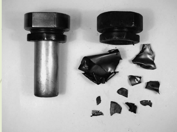
Dry HOBt Koenen-test 10mm
